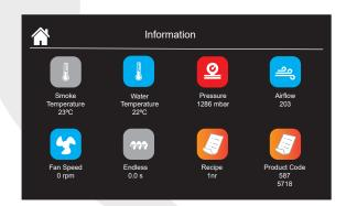
In the reading showed in the previous image, we can see the information offered: smoke temperature, water temperature, pressure, air flow, speed of the smoke extraction fan, working time of the auger, recipe applied to the configuration of the boiler and product code.
