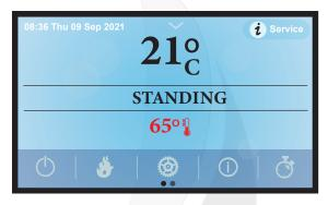
When the message "Service" (Extraordinary Maintenance) appears on the screen, the user must notify a professional or S.A.T. authorized to perform IT, if they have not been recently carried out, the maintenance work that is marked in the table shown below:
