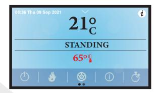
Press the P1 button for a long time, slide to the right and the boiler goes into the process of shutting down until it reaches the state of shutdown.
