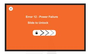
When this message is displayed in the control panel, the boiler is ready to unlock and restart. Slide as indicated on the screen and unlock.
