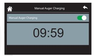
At the first ignition of the boiler, before proceeding to make the ignition, we must make a manual loading of the auger. As shown in the images above, a countdown appears that lasts up to 10 minutes to do the manual loading of the auger. Once the charge has been done, we stop the counter and proceed to the ignition.
